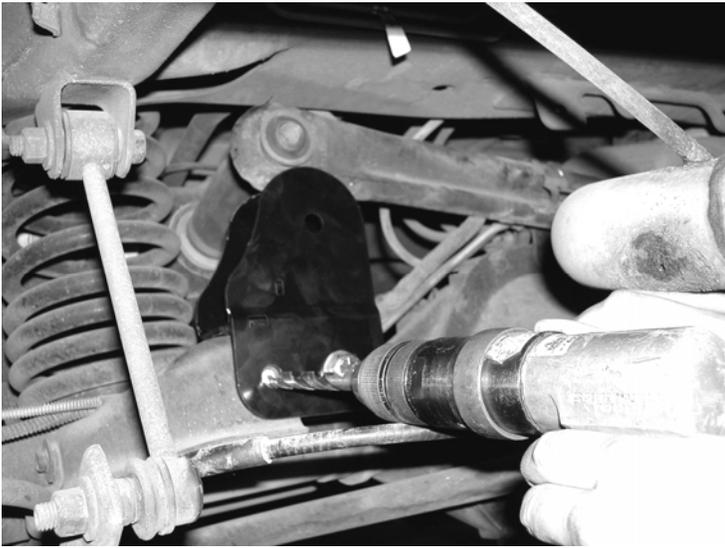
63. Locate the supplied FT1599-2-4 sway bar end links. Install two bushings and one sleeve into each end. Connect the bottom of the sway bar end link onto the sway bar using the supplied 12mm-1.75 x 70 bolts, flat washers and c-lock nuts and connect the top of the sway bar end link to frame with the factory bolt. SEE PHOTO BELOW.
