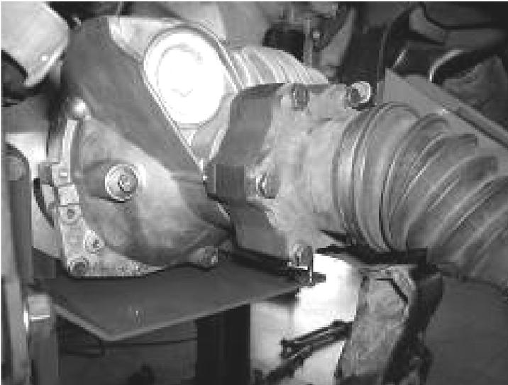
35. Install Fabtech shock part number FTS7191 (not included) using factory hardware. Torque the upper stem bushing to 15 ft lbs and the lower bolt to 35 ft lbs.
