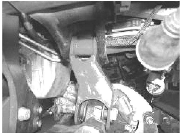
24. Place the differential housing into the Fabtech rear crossmember using the supplied 1/2" x 4 1/2" bolt, nut, and washers along with the supplied large FT55-1 washers attach the differential. SEE PHOTO ON NEXT PAGE.
