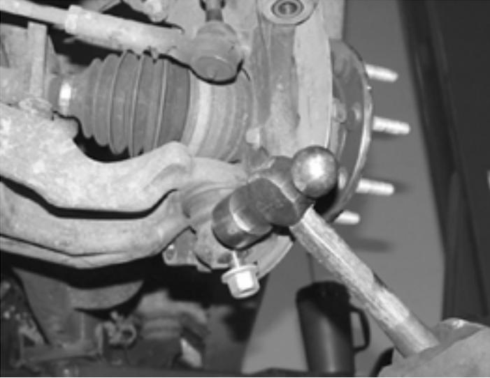
11. Disconnect the CV half shafts from differential housing and remove the axle assembly.
