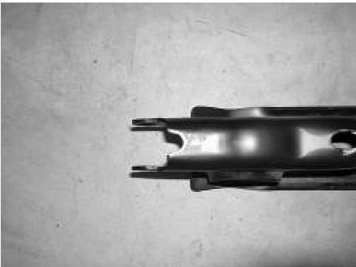
46. Install the factory torsion bar crossmember onto the Fabtech brackets. Note: on some trucks you will need to install the Fabtech torsion bar brackets and factory crossmember as one unit. This will require you to remove the Fabtech bracket after all the holes have been drilled than reinstall as one complete unit.
