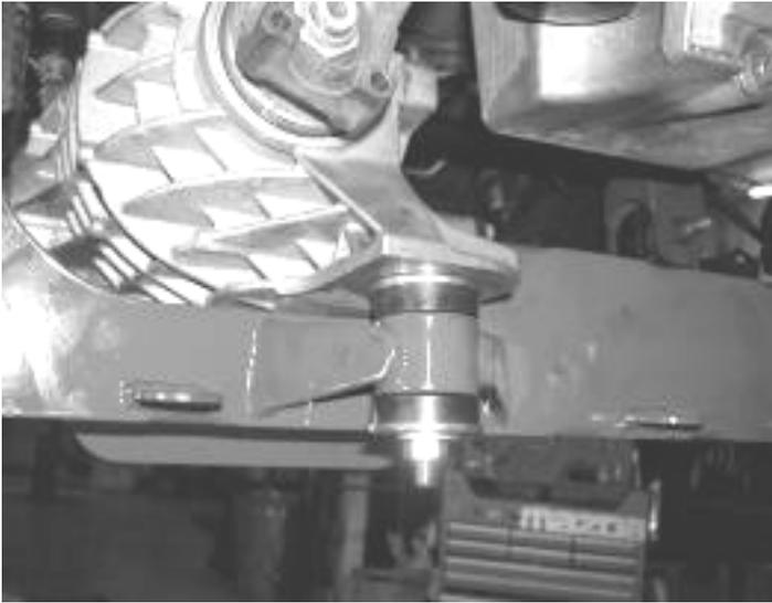
25. Attach the Fabtech front crossmember into the lower control arm pockets using the stock hardware.
