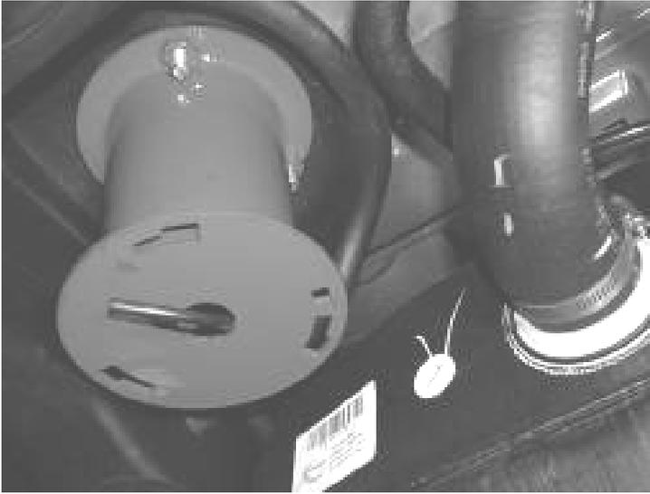
65. Reinstall the factory air bag onto the new spacer previously installed. The air bag will need to be locked into the spacer by engaging the tabs from the air bag to the spacer and twisting the air bag clockwise. Set the lower mount of the air bag onto the axle.
