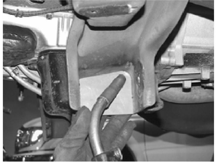
21. Locate and install the Fabtech rear crossmember into the factory lower control arm pockets using the stock hardware with the nuts towards the rear of the truck. Leave loose
