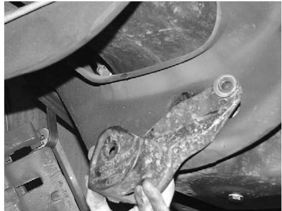
6. Attach the new drop brackets to the frame using the included hardware. You will reuse most of the factory holes and have to drill some new ones. Locate the existing holes with the supplied bolts and mark the new holes that must be drilled with a center punch. SEE PHOTOS BELOW AND ON NEXT PAGE.
